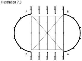
tress posts and on the tension straps. Fix the bearing plate using eight (8) bolts and nuts (BB) 1/4"#20 X 5/8" (6,35 mm X 15,88
