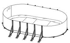
Carefully unfold the liner, bringing the bottom-sidewall seam close to the wall base. Make sure that the side with the protruding seams faces downward or that the patterned side faces upward.
