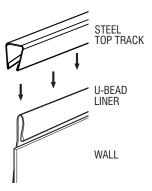
Start the vacuum cleaner to allow the liner to adhere to the wall and check for excess tension at the bottom or for wrinkles. Adjust the liner by removing wrinkles if needed, lift or lower it in order to ensure a perfect fit.
