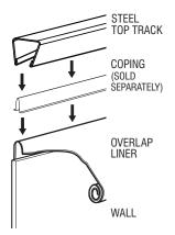
Installation detail of a bead liner with top track.
