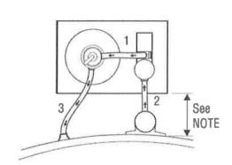
Insert threaded nozzles, if applicable, in order to be able to screw the valve in the skimmer.
