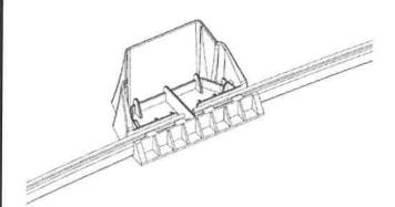
Assemble all bottom tracks to the bottom plates to form a perfect circle with a diameter and a radius in accordance to the chart
