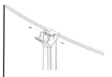
Install the joiner plates on top of each upright then install metal screws at the top of the support posts, making sure the support posts are perpendicular to the ground.
