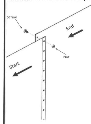
Begin inserting the wall into the bottom wall tracks in the middle of a joiner plate. At first, the wall should be kept in place with one or two support bars (or extra persons). One person should uncoil the wall on a beam or a plank while a second person inserts it in the bottom wall tracks. Do not uncoil more than 3 m (10') of wall before you install a support bar to reinforce the structure.
