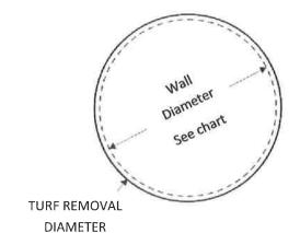
Using a measuring tape, draw a circle 15 cm to 20 cm (6" to 8")longer in radius than the pool, depending on the width of the uprights (See illustration 3.1). Remove all grass from the area that you have outlined.
