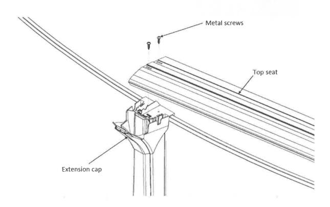
Installthe seat cap to the interior side of the ledge. Secure both (2) parts together by joining the two (2) holes found on the front of the extension cap with the hooks from the leat cap.
