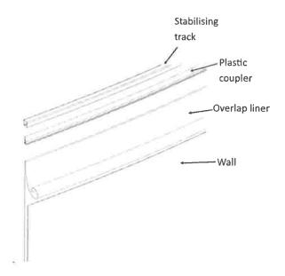
At this point, the liner may be too tight, making it difficult to drape the overlap or, on the contrary, too loose. In such case, you will have to redistribute the tension in the liner by removing some of the couplers and readjusting the liner.
