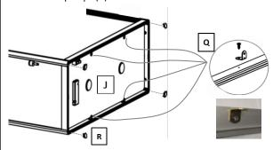
TIP: Thread the power cable through the rectangular hole in the Cover Panel when sliding the Cover on.
