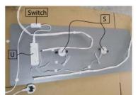
**TIP:** When the light cables are connected, plug the power cable into the mains to test the lights at this stage. Check each connection until the lights are working whilst the cabinet is in this position.
