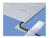
When installing two or more Ambient heating mats next to each other make sure that the heating wires in adjacent mats **DO NOT** overlap. We recommend the use of adhesive tape to ensure that they will not move over a period of time.
