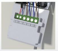
The rest of the thermostat connections can be made according to the instructions with the thermostat and should resemble the picture shown here. Refer to thermostat manual for correct wiring instructions.
