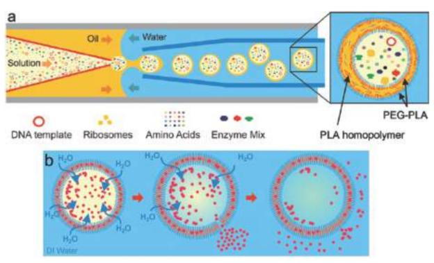
Fig. 26 Protein expressing polymersome GUVs generated by microfluidics. Schematic representation of (a) the methodology used to generate these artificial cells and (b) protein release under osmotic shock and subsequent self-sealing. PEG: poly(ethylene glycol). PLA: poly(lactic acid). Reprinted with permission from C. Martino, S. H. Kim, L. Horsfall, A. Abbaspourrad, S. J. Rosser, J. Cooper and D. A. Weitz, *Angew. Chem., Int. Ed.*, 2012, **51**, 6416–6420. Copyright (2012) Wiley.<sup>243</sup>
