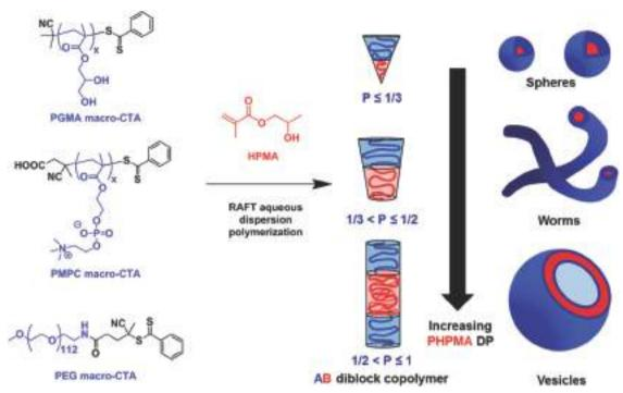
Fig. 8 Polymerization-induced self-assembly (PISA) of 2-hydroxypropyl methacrylate (HPMA). A variety of macromolecular chain transfer agents (CTAs) were used to produce various assemblies depending on the degree of polymerization of HPMA. Reprinted with permission from N. J. Warren and S. P. Armes, J. Am. Chem. Soc., 2014, 136(29), 10174-10185. Copyright (2014) American Chemical Society<sup>68</sup> (https://pubs.acs.org/doi/abs/10.1021/ja502843f)
