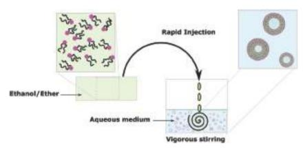
Self-assembly of lipids and block copolymer vesicles by using solvent injection.
