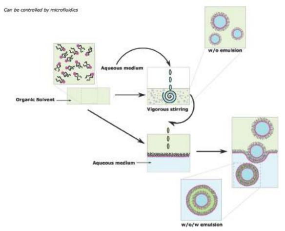
Fig. 10 Self-assembly of lipids and block copolymer vesicles by using emulsion phase transfer.
