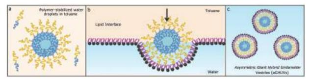
Fig. 18 Preparation of asymmetric hybrid GUVs by emulsion-centrifugation. (a) Preparation of sucrose filled polymer-stabilized droplets in toluene. (b) Crossing the amphiphile-stabilized glucose/toluene interface helped by centrifugation, forming (c) asymmetric hybrid vesicles. Adapted from A. Peyret, E. Ibarboure, J.-F. Le Meins and S. Lecommandoux, Adv. Sci., 2017, 5(1) with permission from Wiley. (https://onlinelibrary.wiley.com/doi/abs/ 10.1002/advs.201700453).87
