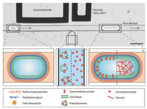
Fig. 12 Sequential bottom-up assembly of transmembrane and cytoskeletal proteins into droplet-stabilized GUVs by high throughput pico-injection. Scale bar 50 μm. Reproduced with permission from M. Weiss, J. P. Frohnmayer, L.T. Benk, B. Haller, J. W. Janiesch, T. Heitkamp, M. Börsch, R. B. Lira, R. Dimova, R. Lipowsky, E. Bodenschatz, J. C. Baret, T. Vidakovic-Koch, K. Sundmacher, I. Platzman and J. P. Spatz, *Nat. Mater.*, 2018, 17, 89–96.
