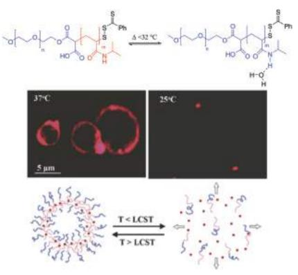
Fig. 15 Thermoresponsive block copolymer bearing the thermosensitive PNIPAM block with LCST behavior. Reprinted with permission from S. Qin, Y. Geng, D. E. Discher and S. Yang, *Adv. Mater.*, 2006, **18**, 2905–2909. Copyright (2006) Wiley. 148
