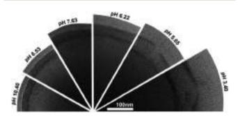
Fig. 14 Cryo-TEM image of a pH-responsive PEO-b-PS-b-PDEA polymersome at different pH values. Reprinted with permission from S. Yu, T. Azzam, I. Rouiller and A. Eisenberg, J. Am. Chem. Soc., 2009, 131(30), 10557-10566. Copyright (2009) American Chemical Society. 138
