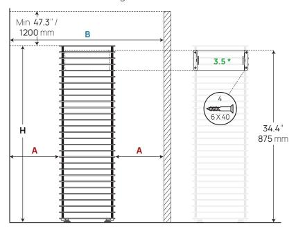
\* CLIFF Mini 3.5 is attached to the wall with a special bracket See CLIFF Mini 3.5 heater data in the table below.
