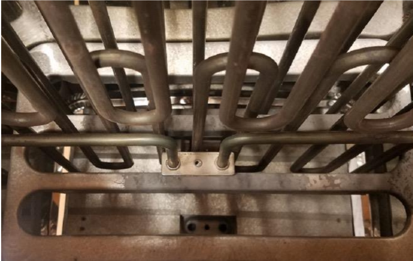
IMAGE 5 - Stand heater upright & gently pull/wiggle unsecured element out of the body of the heater
