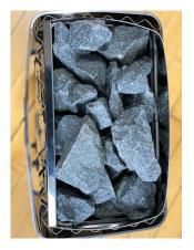
Note: Packing stones in too tightly will restrict airflow and affect the efficiency of your heater. Loosely position the stones around and above the heating elements. It is common to have 5-10 stones left over.
