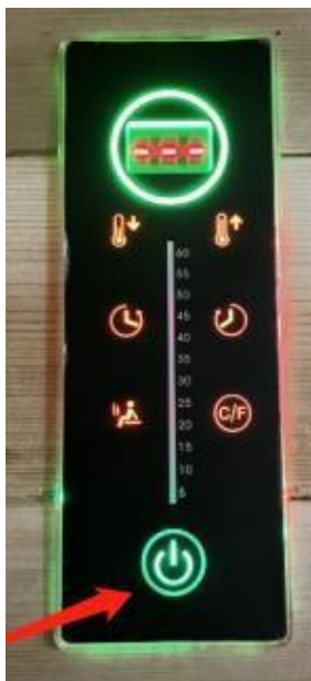
Sauna Control Panel is Illuminated
