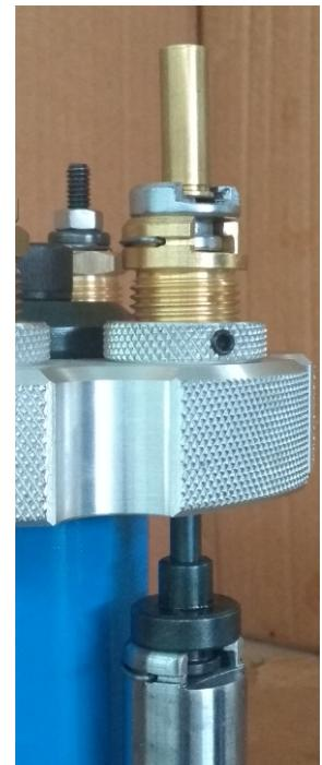
**2. PRIMING:** Die # 2 - removeshell holder from piston and drive it on priming die. Place priming pin and base in piston end drive it up to the end of travel. Place a primed case on shell holder whitch is on die and screw it until touching the pin. Fasten its conternut and fixe the bolt.
