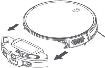
3.2 Press the switch of the dust box of the water tank, open the dust box and pour the garbage into the trash can.
