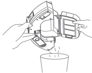
3.3 Remove the filter gauze/ HEPA and sponge, and clean the filter gauze with water. Use a cleaning tool to remove debris from the HEPA. HEPA can't be washed, sponges can be washed. Then clean dust box, waiting for the sponge and filter gauze were to dry up again after use.
