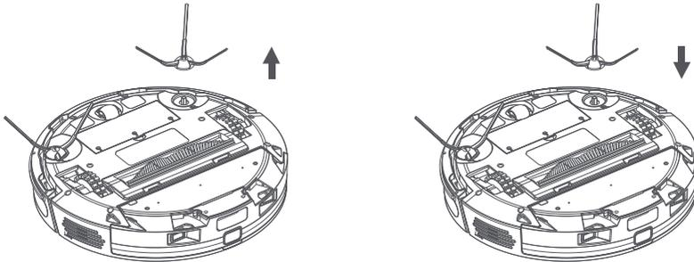
\*Match left-side brush (L) and right-side brush (R) with the letters L and R on the bottom case, respectively and press down to install it.
