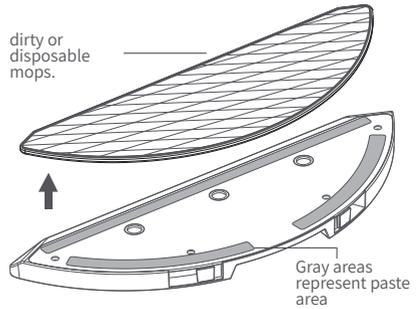
4.3 Clean mop or disposable mop clean and dry, to install or remove a new mop, disposable mop mop stents. Finally, install it back to the robot in the opposite direction of the removed bracket.
