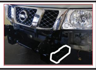
• Bolt Up all nuts using genuine nuts from the vehicle Or nuts and bolts provided (do not tighten all the way, keep enough to allow slight movement) this will be tightened at a later stage.
