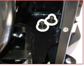
• Use protection plate L shaped brackets to mount the protection plates.
