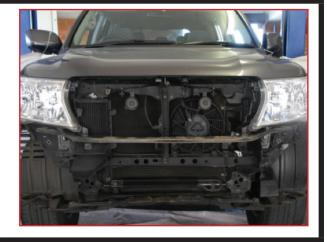
Remove cross section support
