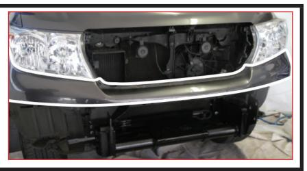
• Once the bulbar has been unwrapped place the bar on the vehicle resting on the mounting bracket – NOTE if you are mounting a winch, this has to be done prior to mounting the bulbar on the bracket.
