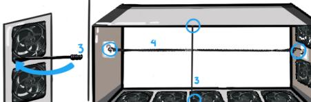
5) Attach 4 top fan cables to the 5-way fan hub. Note tongue & groove make 3-hole plugs fit only one way into 4-pin sockets!
