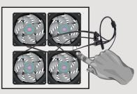
Each corner of the fan should be flush with the underside of fan plate. Carefully tuck fan cables between fans and secure with zipties through the holes in back of fans. Make sure cables cannot stray into fan blades.
