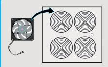
Flip the fan panel over and arrange fans over pins with printed specs on fan hubs facing the fan grills. Holographic stickers will face into the assembled box so fans blow outward.
