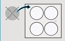
Place fan grills over the precut holes (raised side faces outwards) on what will become the top panel of the Brisk Box.
