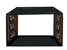
4) Hook or tie the bungee between opposite sides using back screw holes of middle fan. Tension slightly so panels bow inward a bit.
