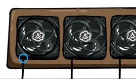
3) Screw together the side fan panels and black bridge panels.
