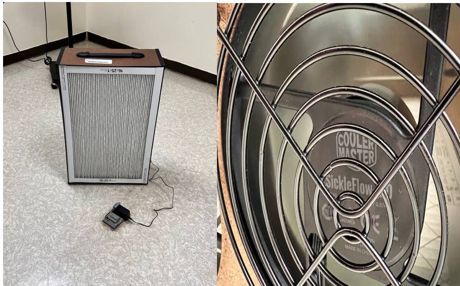
Unit in Test – Sickieflow Fans – 5 Fan Configuration
