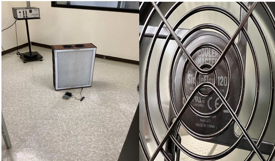
Unit in Test – SickelFlow Fans – 7 Fan Configuration
