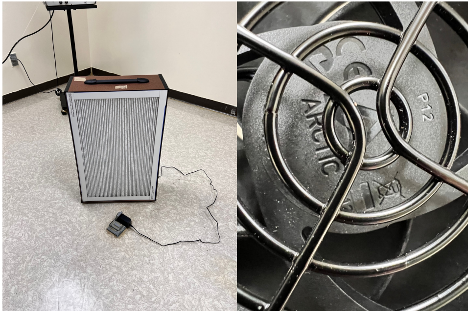
Unit in Test – Arctic P12 Fans – 5 Fan Configuration
