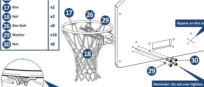
Note: After installing the (#17) Rim, attach the (#18) Net, making sure the longer strands are on top. If the net is not attached properly, scoring can be affected.
