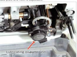
tank and oil wick lubrication mechanism.
