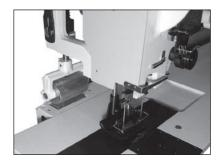
Clutch driven puller feed
