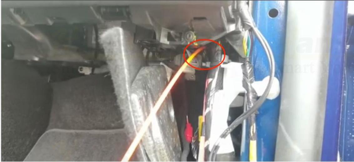
9. Once the fish tape is visible from the passenger side, pull it inside
