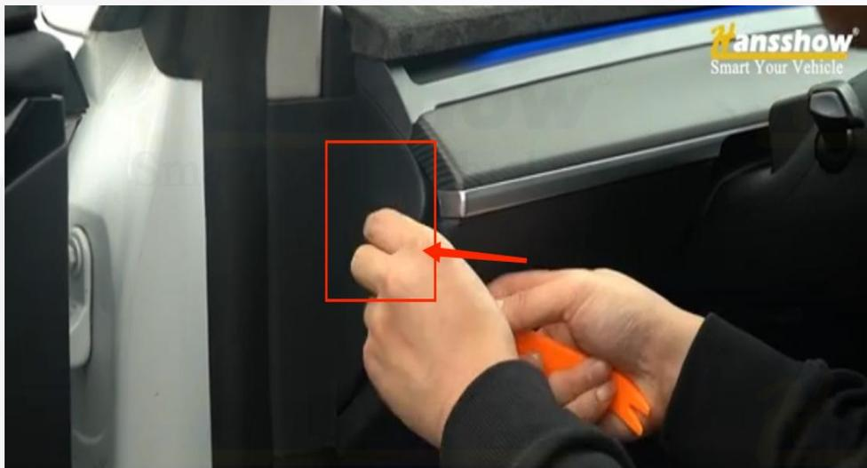
1. Use a pry bar to pry open the left and right small side panels.
