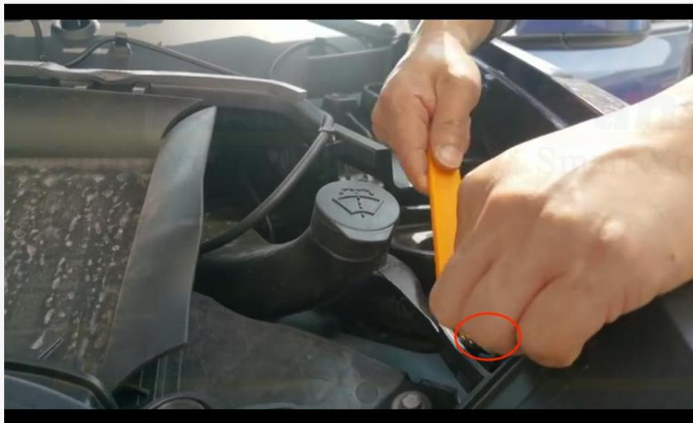
3. After removing the cover plate, take out the retaining clip.
