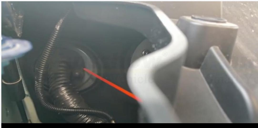
8. Thread the fish tape from the rubber plug near the air conditioning vent into the driver's seat.
