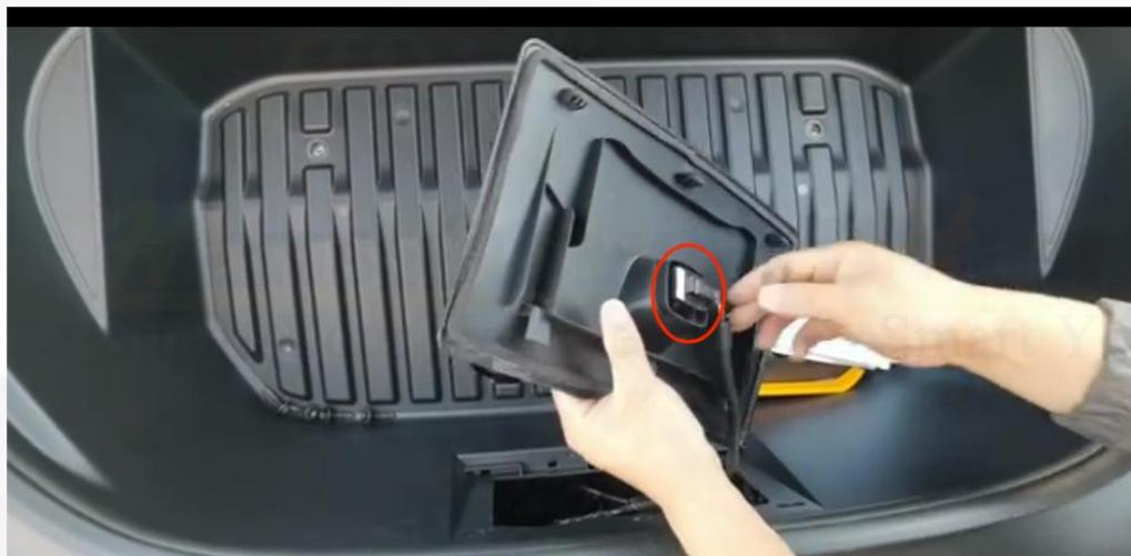
4. After unplugging this connector, remove the Frunk cover
