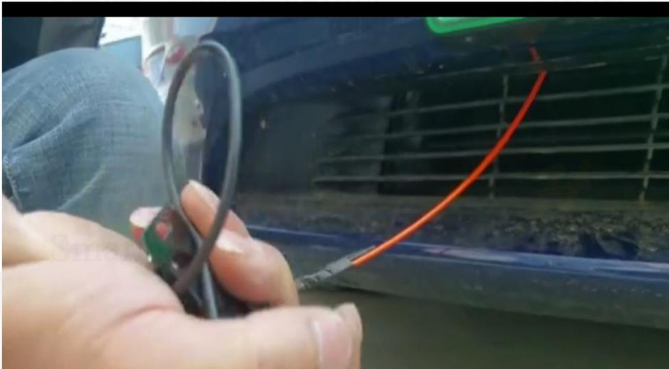
6. Wrap the camera cable around the fish tape and thread it into the engine compartment.
