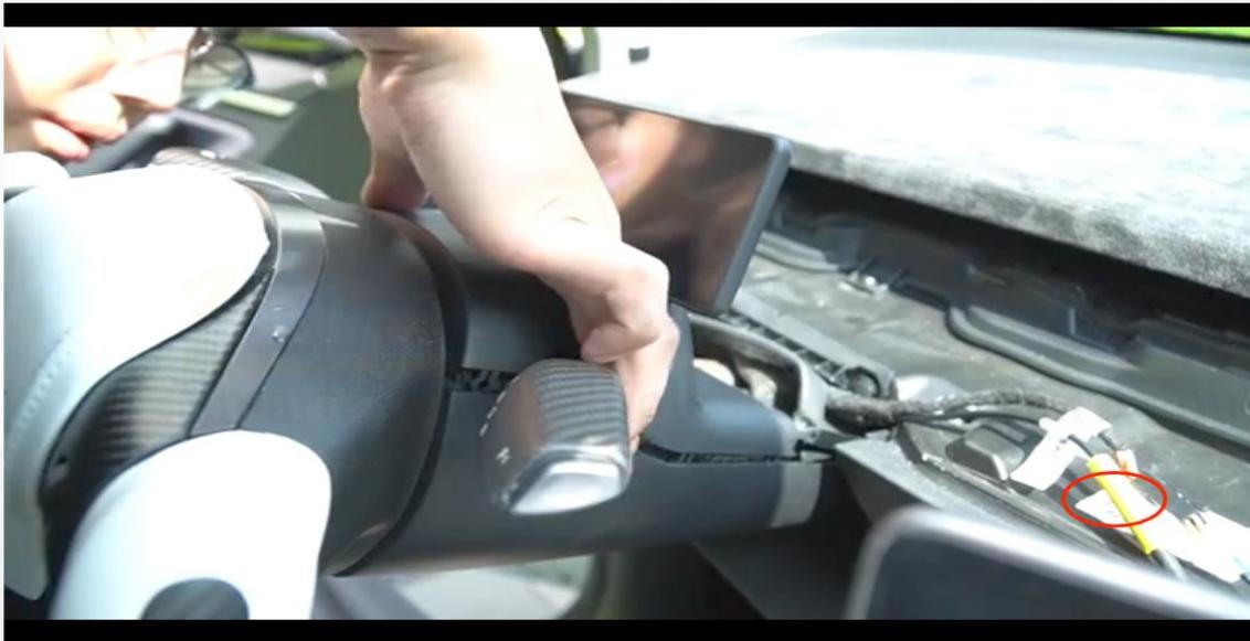
10. Connect the camera cable and route it along the wood trim panel. Once the wiring is in place, restore the vehicle to its original condition.
