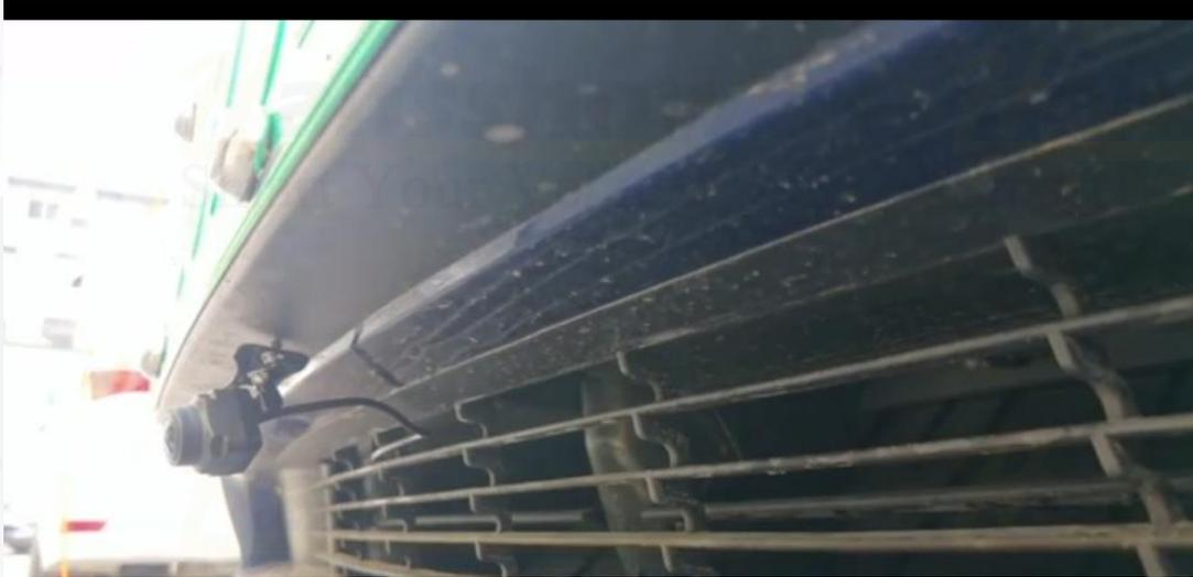
7. Install the camera bracket in the correct position and tighten the screws once it is aligned properly.
