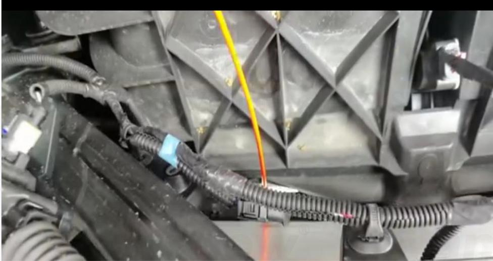
5. Start routing the wires by using a fish tape to thread the wires from the grille below the license plate into the engine compartment.
