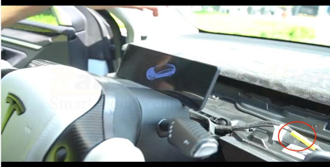
5. Use a pry bar to pry open and remove the original cover plate from the indicated position in the image. Then, install the instrument screen in its place.
