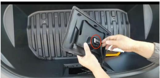
3. After removing the cover plate, take out the retaining clip.
