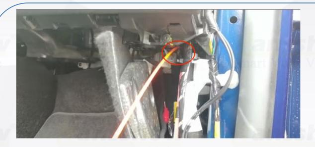
9. Once the fish tape is visible from the passenger side, pull it inside
