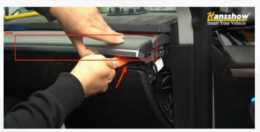
1. Use a pry bar to pry open the left and right small side panels.
