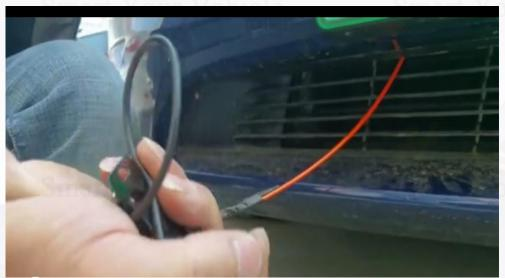
5. Start routing the wires by using a fish tape to thread the wires from the grille below the license plate into the engine compartment.
