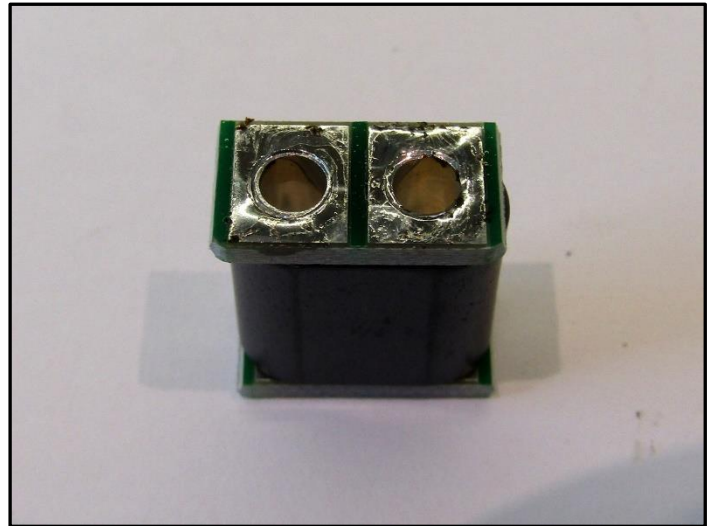
Figure 5d: Fully assembled transformer.
