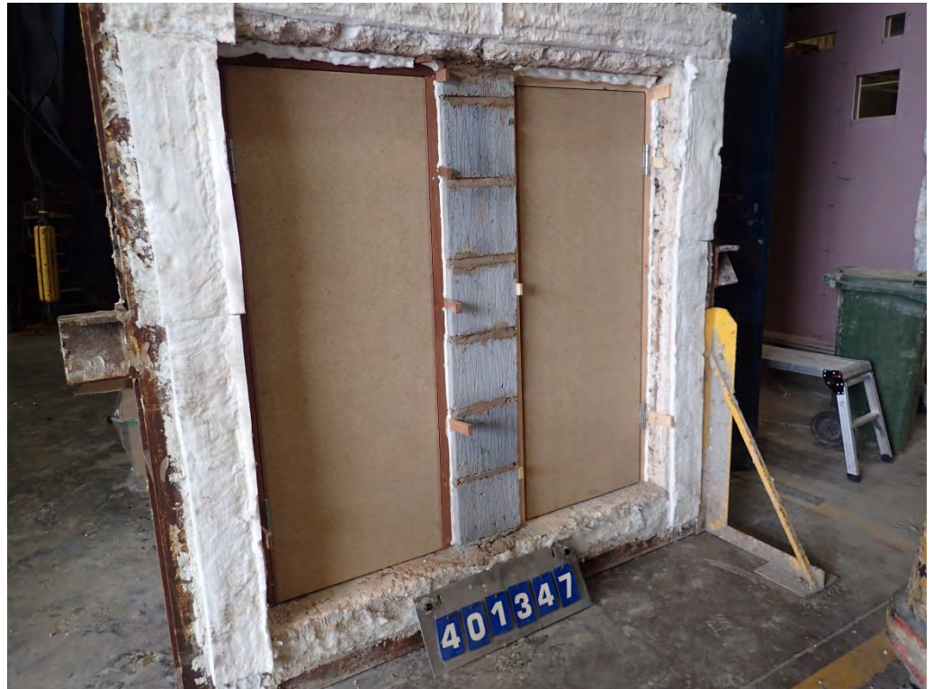
The exposed face of the doorsets prior to the start of the test
