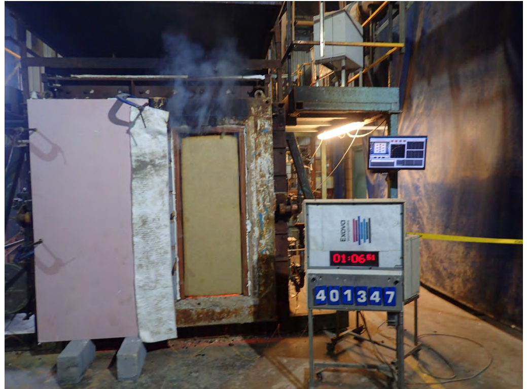
The unexposed face of Doorset B after a test duration of 66 minutes
