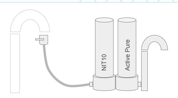
**Filter Order Matters:** Place the Nitrate Filter in the first Sump and the Active Pure Filter in the second
