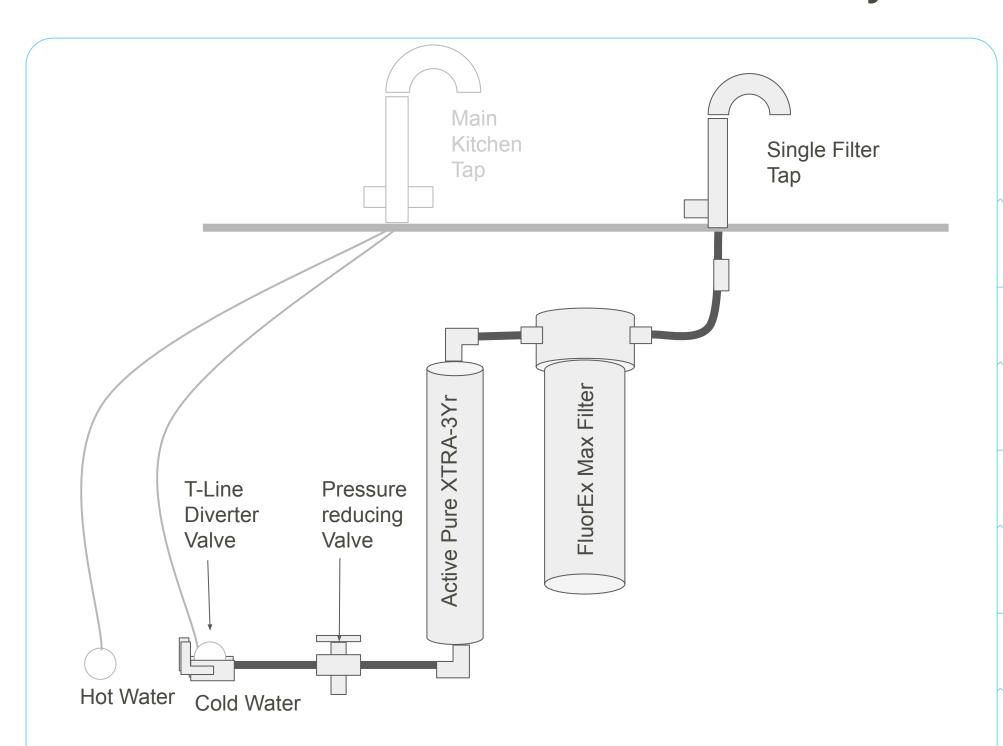
Establish position for the tap on the sink and drillan appropriate sized hole. Install the T-line diverter valve into the cold water line. Install pressure reducing valve upstream of the filters. Install the Filters in the order shown in this diagram
