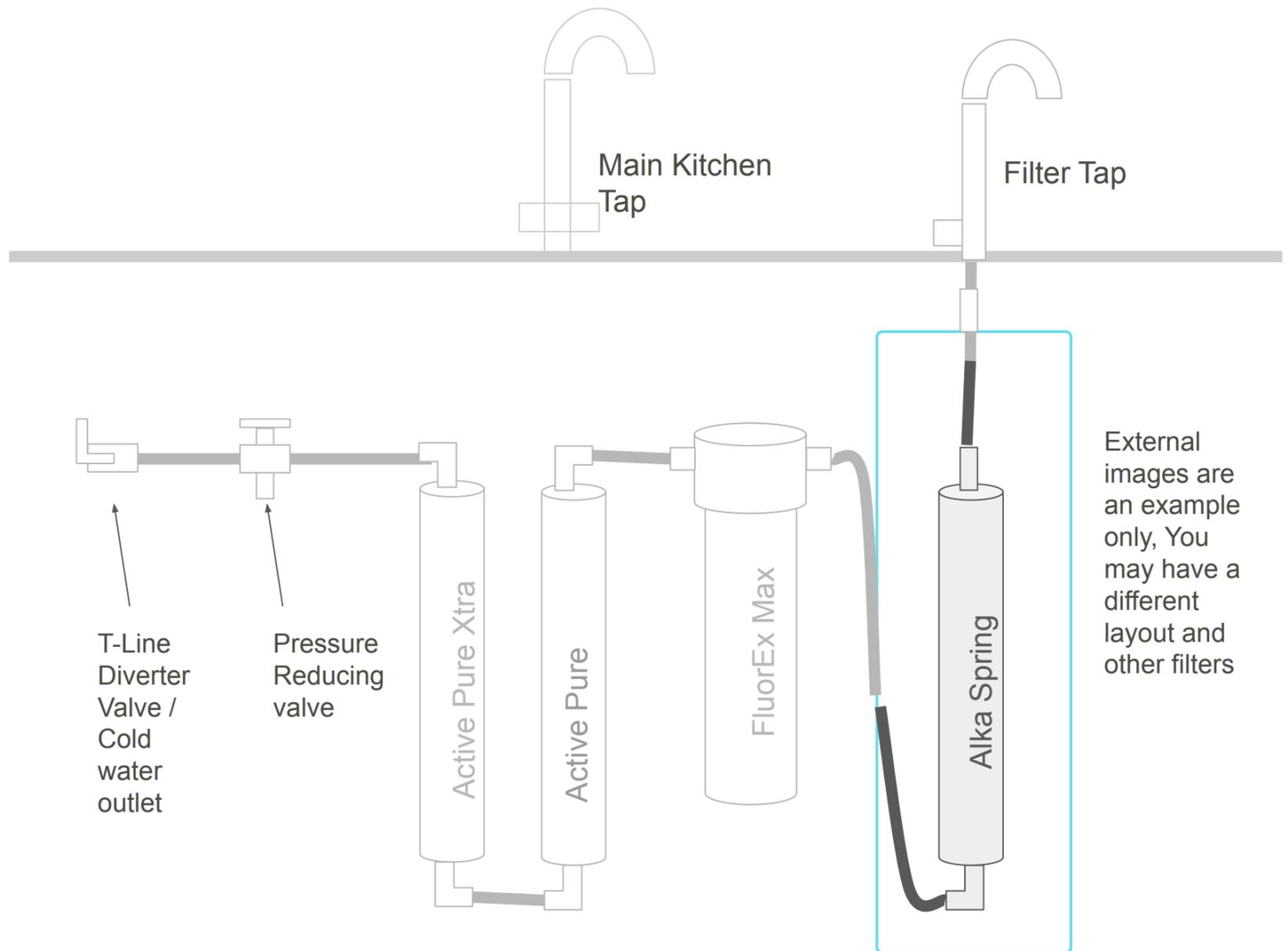
The Alka Spring should be downstream/after any filters in your existing water system, and before any ionizer.
