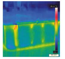
Heat leak test performed with the Nordic Insulation System
