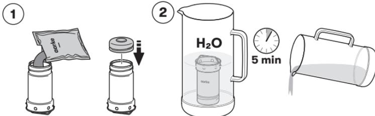
1. Add the filter granules to the filter cartridge. Close the filter cartridge lid.
