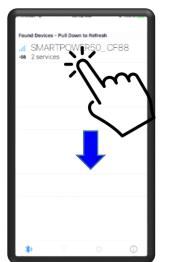
To re-scan or refresh the list of available nearby SMARTPOWER 50 devices, pull down on the middle of the screen and the app will re-scan for devices for another 2 seconds.
