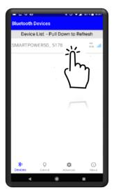
Once the desired SMARTPOWER 50 device appears on the screen, it becomes available for Bluetooth connection. To connect to the SMARTPOWER 50 device, click on the banner containing the SMARTPOWER 50 device's unique ID.
