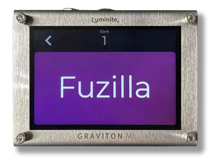
Live screen is optimized for live performance with the super-sized **Preset** name that can be read across the stage. All touch screen buttons are disabled except the < (back) button to prevent accidental changes while performing.
