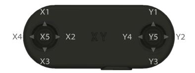
Each EC Controller has two rotary encoders, each can be pushed down as a button.
