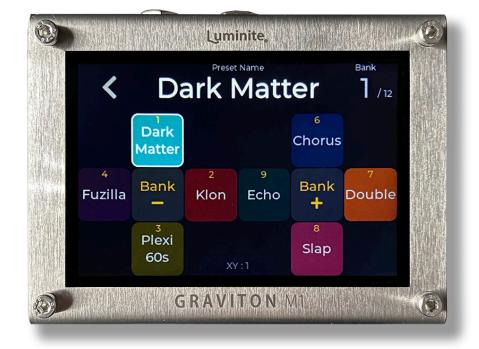
This Screen is for assigning the **XY Controllers** switches to the designated **Presets** / **Actions**. The last activated switch is highlighted.
