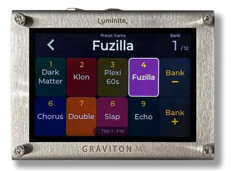
This Screen is for mapping the 6 x built-in **Footswitches** (M2) or external **Footswitch Pedals** to the designated **Presets** / **Actions**. The last tapped footswitch is highlighted. If a **Lumnite F** Series Footswitch is used, the **Block** layout will match with their physical layout automatically.
