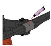
Install the handlebar in the same plane of the stem with the desired handlebar angle.
