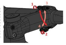
Align the cockpit with the front wheel in such Tighten the top cap screw until no more play. Tighten the steerer screws in such a way that the same plane.
