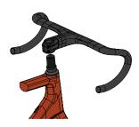
on the stem steerer side of the barstem (ti-prep for titanium bolts) and tighten the fixing screws until reaching the **5.2 Nm** In ¼ turn 5.2 Nm increments, please remember to slowly tighten the bolts on the steerer clamp evenly to ensure even load distribution.
