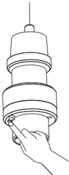
1. Press the program button on the receiver for 6 seconds until the indicator light starts to flash rapidly. (Note: The light flashes from slowly to rapidly.)
