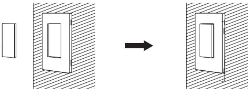
4. Attach the transmitter to the base.
