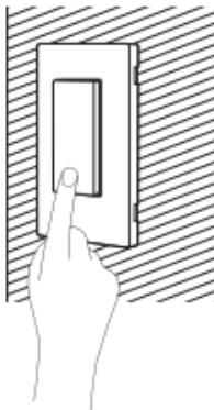
5. Press the ON/OFF button on the wall switch remote control to turn the receiver on and off.
