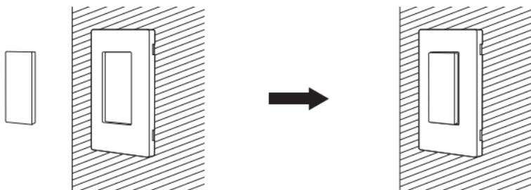
4. Attach the transmitter to the base.
