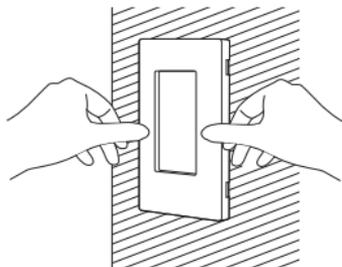
3. Attach the upper shell to the lower shell.
