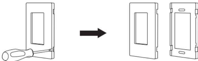
1. Separate the upper and lower shells of the Wall Switch.
