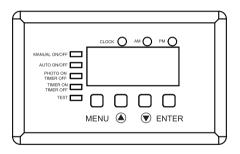
**MANUAL ON/OFF** - Press the button to select ON, the transformer will be on all the time. Press the button to select OFF, the transformer will be off and the lights will be off.
