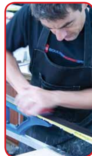
5-Polish with nylon by brushing with high pressure, back and forth.
