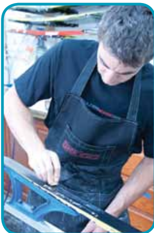
Applying solid fluoro block
