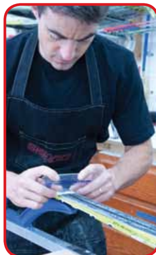
3-Once the ski has cooled, lightly scrape excess powder off the base.
