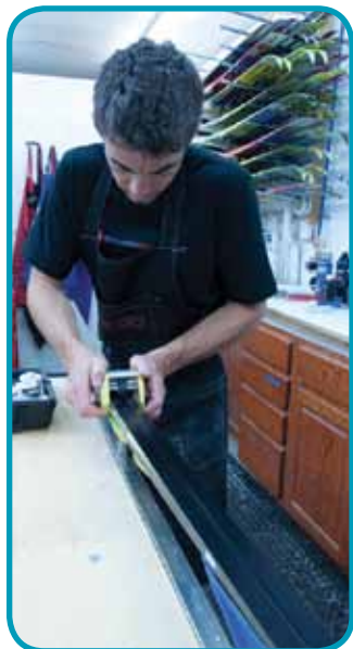
Applying hand structure.
