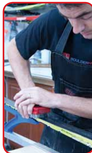
4-Use a metal or horsehair brush to remove additional excess material from the base.
