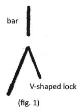
View the instrument head-on, with the beaks pointing toward you. You should now see the two parts of the locking mechanism: a flat, rectangular **bar** and a **V-shaped lock** portion.
