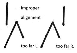
If the two mechanisms do NOT line up as stated, you can bend the bar back into proper position with your thumb so that it aligns with the V-shaped lock portion a shown in fig 2.
