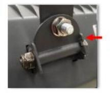
Heater bracket installed outside upper tab.
