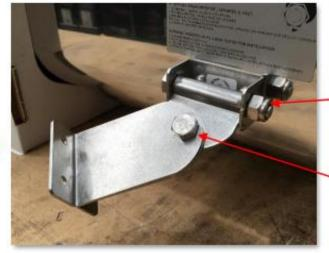
Tighten heater bolt to lock heater at desired angle.
