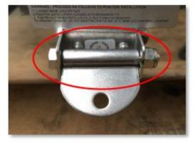
Heater bracket is bolted to the mounting bracket with the supplied short M8 bolt (use 13 mm spanners).
