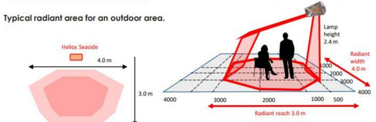
For an open outdoor area with no roof, radiant output is reduced.
