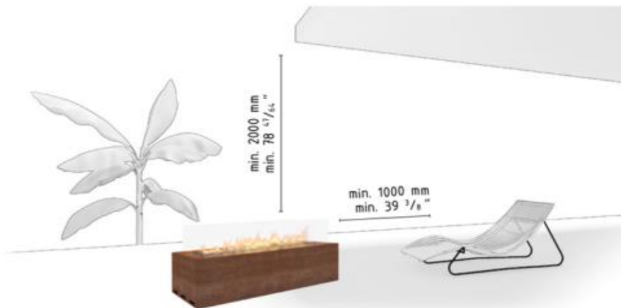
Figure 1: Minimum distance to flammable materials
