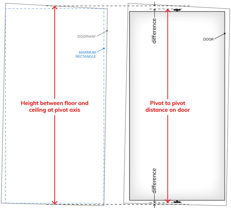
Compare the measured doorway height at the pivot axis with the pivot to pivot distance of the door. Synchronize them if necessary by using one of the hinge height adjustment options on the next page.
