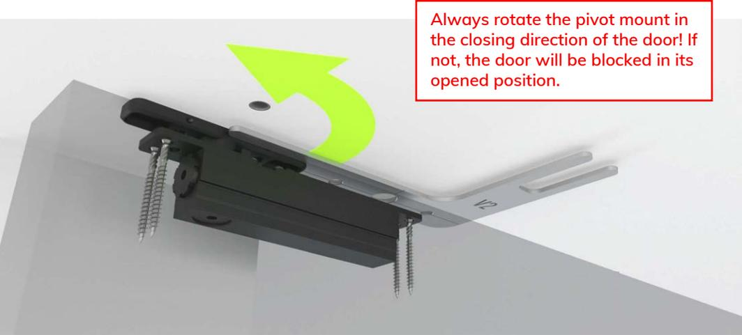
Always rotate the pivot mount in the closing direction of the door! If not, the door will be blocked in its opened position.
