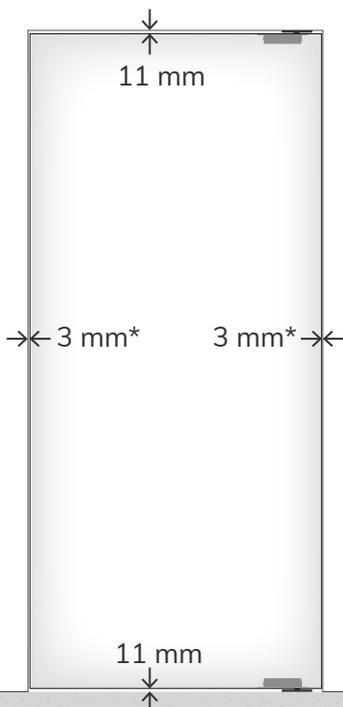
**Top & bottom joints:** min. 11 mm
