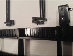
1) Connect part(A) to both sides(B) into 3rd hole from top. Push down to lock. The longer legs of the sides must be facing forward to prevent display from toppling forward from product being displayed. Ensure that the sign tabs(C) are facing upward and the grooves shown in above right picture and facing rear.
