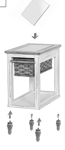
**NOTE:** Feet are labeled (A, B, C, and D) and should be installed in their corresponding places (corners)
