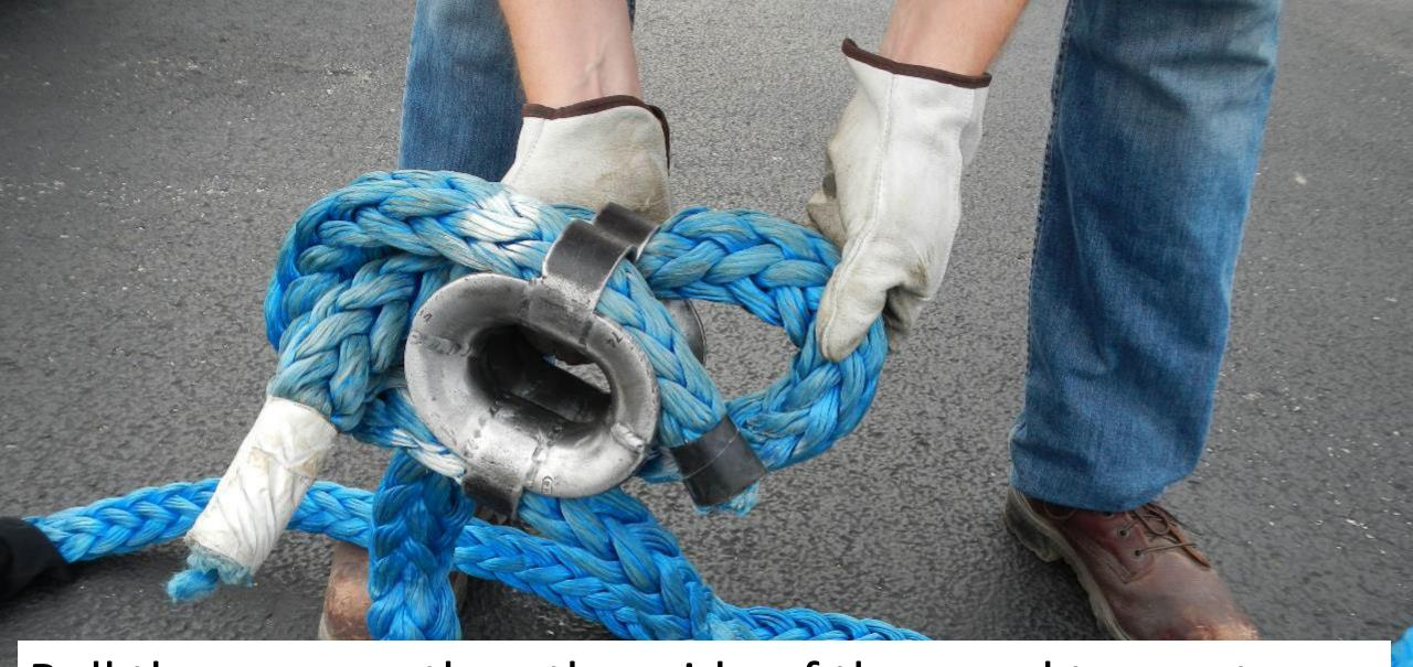
Pull the rope on the other side of the spool to create an opening.
