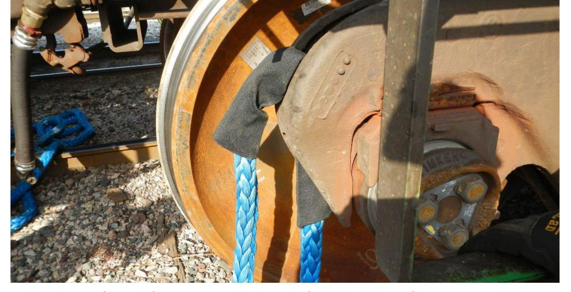
Ensure that the protective sleeve on the tow rope is properly positioned in the side frame.
