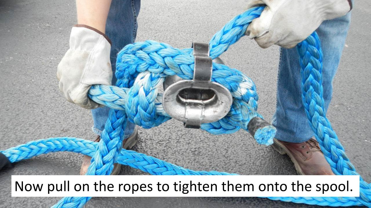
The picture below shows how the rope and tails look when properly threaded through the spool.
