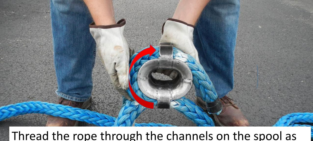
Thread the rope through the channels on the spool as shown, leaving an 8 inch or more tail. Both tails on the spool should be about equal in length.
