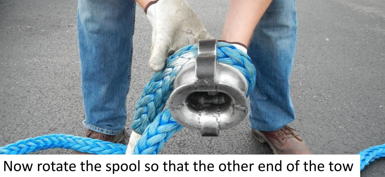
Now rotate the spool so that the other end of the tow rope can easily be threaded through the other side of the spool.
