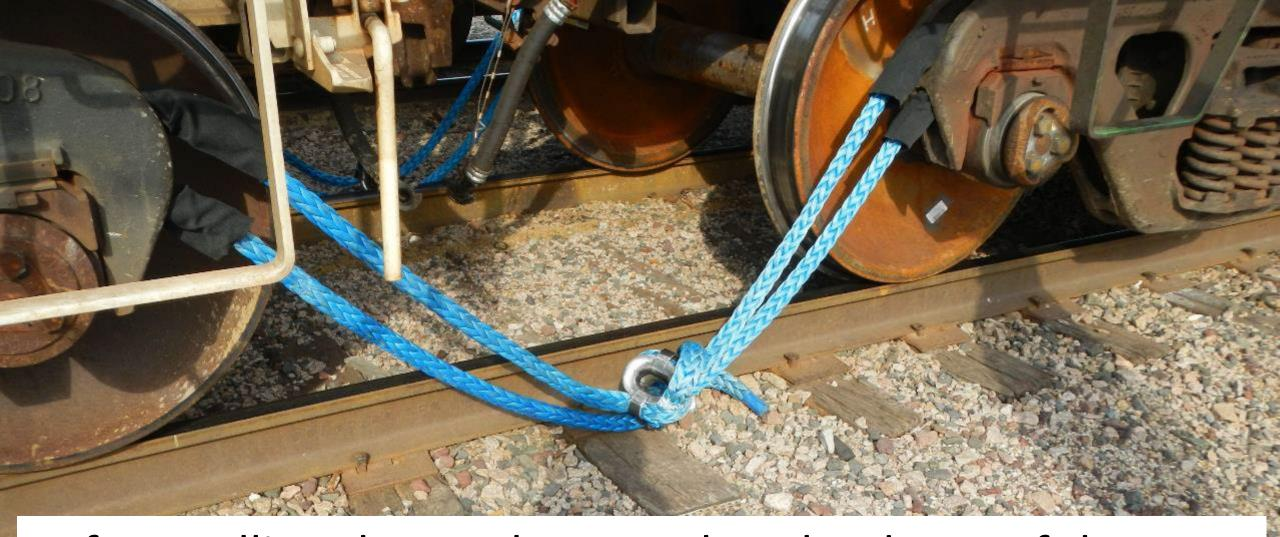
Before pulling the car, be sure that the drape of the tow ropes on both sides of the railcars is about the same.
