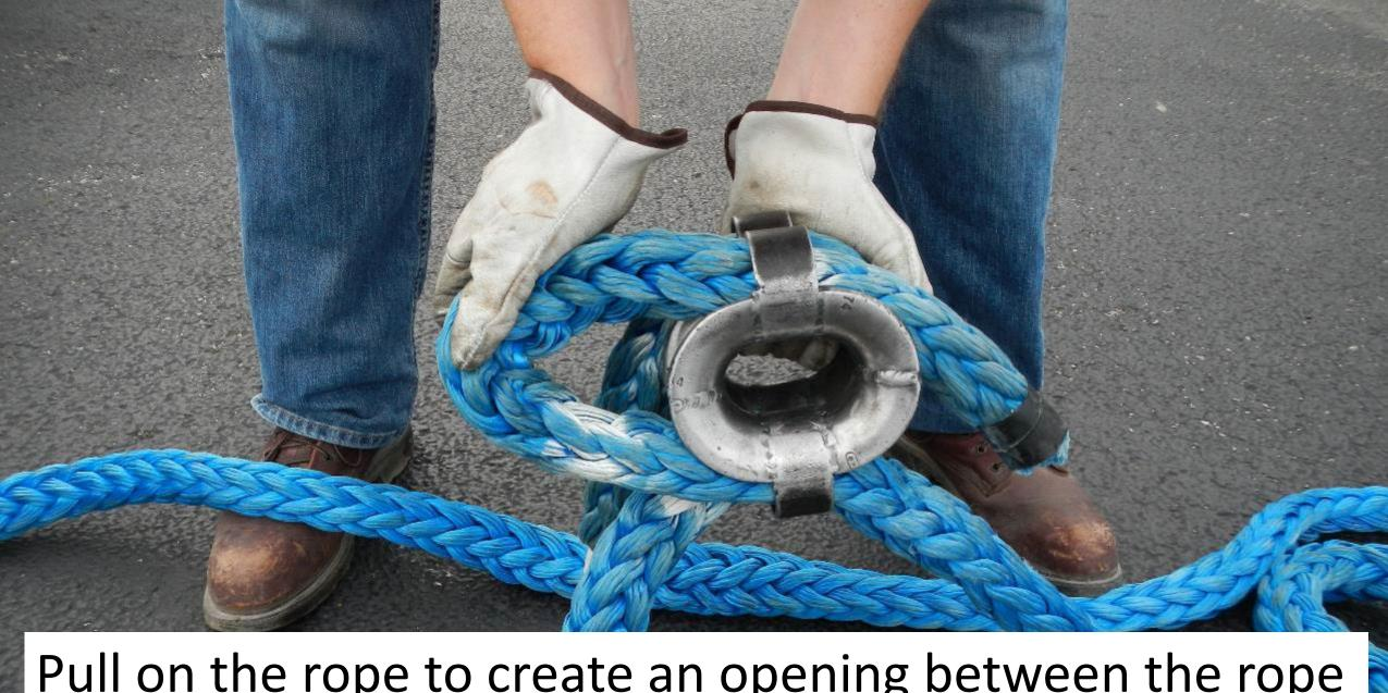
Pull on the rope to create an opening between the rope and spool.
