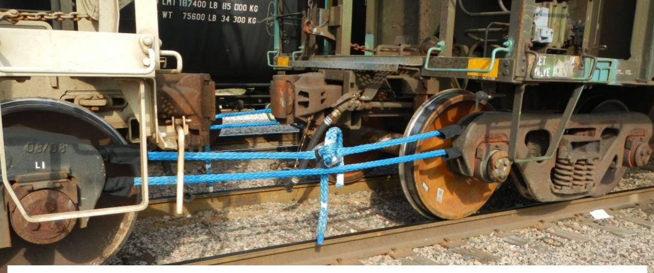
Here both tow ropes are stretched before actual towing begins. Notice that the rope on each side looks equal in tightness.
