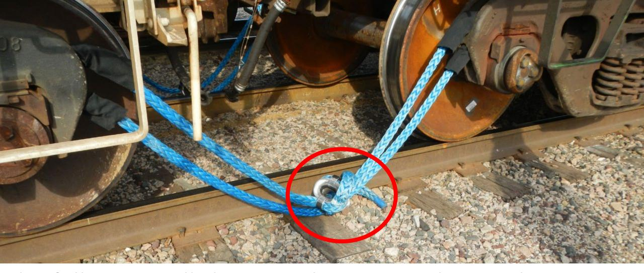
The following will show you how to tie the two loose ends of the rope together onto the metal spool so that it looks like the photograph.
