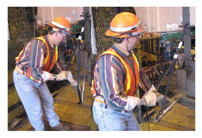
To release the lifter, press on mechanism and pull
