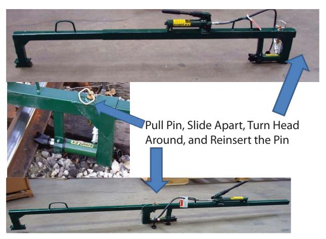
Pump Handle a Few Times To Make Sure the Unit is Tilted So Pressurize the System Fluid is in the Head
