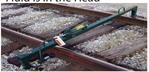
Check to Make Sure "V" Block is Fully Threaded to Cylinder Before Using
